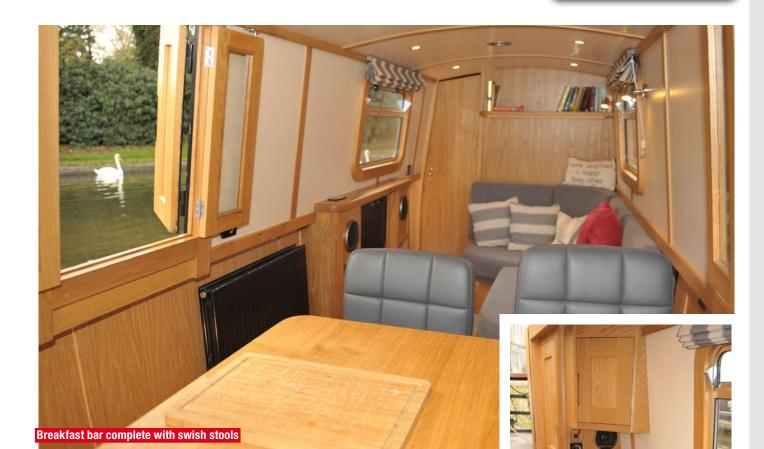
you pass through the galley. There is some great joinery on show, with a beautifully curved door at the end of the run of units. Behind, tucked under the gunwale, is a pull-out wine rack - complete with the outline of a bottle inlaid in a darker wood. There's also a pull-out spice rack.
